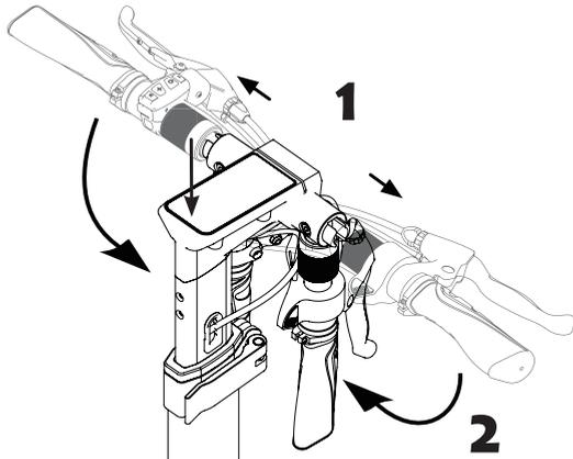
2 To fold QUICK<sup>4</sup>, release the **RED SAFETY LOCK** first, push the steering bar firmly forward while at the same time using your foot to push the **RED** pedal down to release the FOLDING MECHANISM
