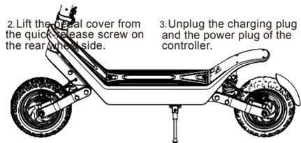
2. Lift the pedal cover from the quick release screw on the rear wheel side.
