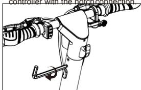
3. Align the T-bar of the scooter then insert it into the pole, use the screw provided with the scooter to install and fix it.
