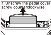
1. Unscrew the pedal cover screw counterclockwise.
