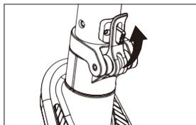
1. Unfold the pole and fasten the folding lock.
